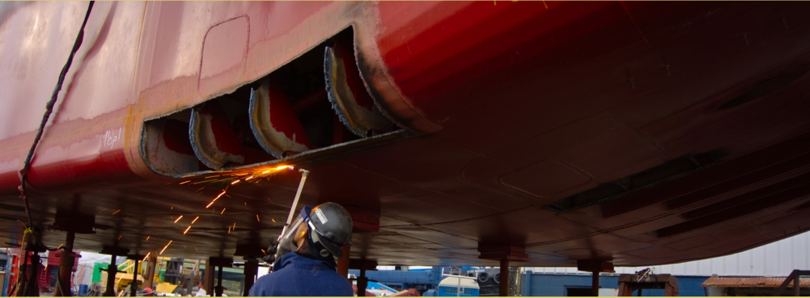
Paint removal for welding pathways enabling hull improvements.
